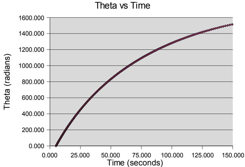
From there I used numerical differentiation to obtain the speed. However, instead of using the nearest neighbours technique I calculated the slope of the line passing through seven data points. The central data point and the three on either side. The reason I did it that way is because the time between data points was exceptionally small and therefore the error in using the nearest neighbours method was large. Here is the result from processing the data in the above graph.
