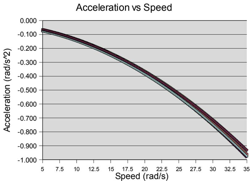
Next, I added four Schwalbe plastic rim strips to the wheel and took five more sets of data. The added mass was  $84.0 \pm 0.5$  grams (as weighed on a digital scale, Salter model 2001, uncalibrated) placed at  $0.312 \pm 0.0005$  meters. This works out to an added MoI of  $x = 0.00807 \pm 0.00005 \text{ kgm}^2$ . Five more sets of data were taken. After crunching the numbers as above, we get these results.
